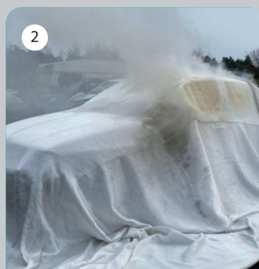
2930-96 Fire blanket lithium battery risk.
